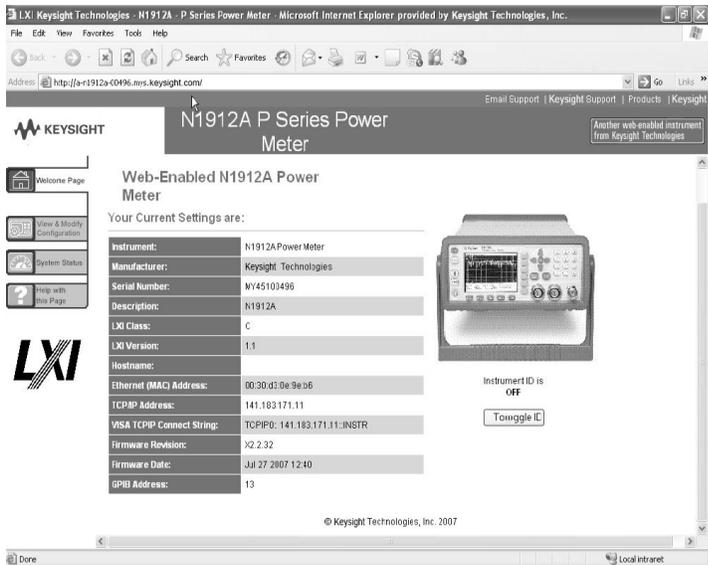
Figure 2. Instrument web page browser that provides instrument's setting at a glance and enabling remote access/control.
